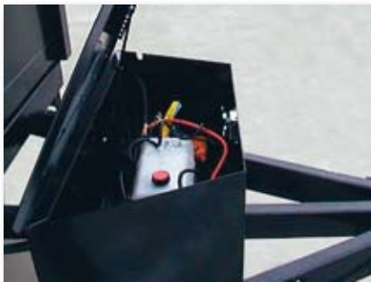
Hydraulic Power Unit/ Battery Storage Box
